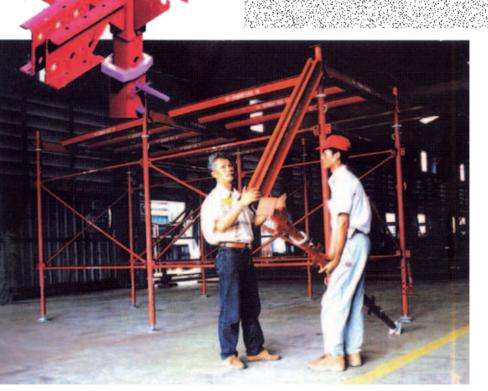
The ends can also be tilted to allow casting of angled slabs in tunnel situations. This system is made to cast heavy concrete slabs and beams.
