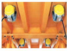
The frequency can be set (from 0 to 9.000 vibrations) when used in combination with an adjustable frequency inverter. This feature minimizes sound emissions as well as increasing consolidation performance.
