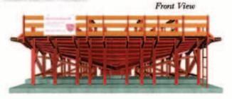
Typical Formwork for Precast Type 1A
