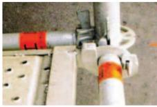
Just one hit of a hammer on the wedges is sufficient to obtain complete stability & safety of the connecting components.
