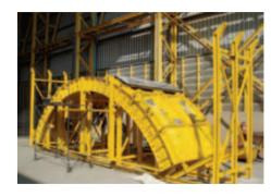
The main sources of strain being; the builtin vibrator system, which helps to vibrate the concrete during the casting stage & are the numerous casting operators and handlings systems sustained by the mould; in order to produce thousands of segments needed to construct each tunnel.
