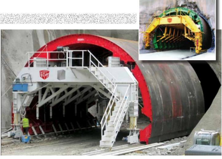
FULL ROUND TUNNEL FORMWORK SYSTEM for PIPELINES Telescopic, "full round" multi-section formwork ideal to achieve continuous advancement or block jets. Self-propelled, hydraulic transport carriage available in the traditional version come with all accessories, such as pneumatic or electric side-wall vibration, jet spray system with articulated feed piping, service carriages, concrete mixing trains.
