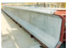
Pre-stressing is a technique introducing stresses to the pre-determined magnitude into a structural member; to improve its behavior. This technique is usually found in concrete beams, spandrels, columns, single and double tees, wall panels, segmental bridge units, build-tee girders, & I-beam girders etc.
