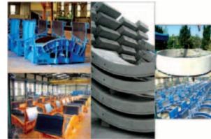
A segment mould is composed by a Soffit part, Four (4) Side Form and Two (2) Top Panels.
